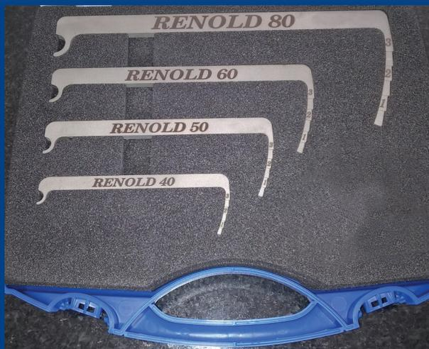
The Renold Chain Wear Guide makes inspecting chain elongation quick and easy. It measures chain elongation caused by continuous running, without removing the chain from its installation location. Chain should be replaced before elongation reaches 3 percent to prevent the chain from jumping over the sprocket teeth. Save costs by avoiding premature sprocket wear and eliminate the complicated, time-consuming process of removing and re-installing chain required by conventional testing methods.
