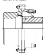
Coupling with long boss inner member and large boss driving flange: Increases shaft engagement and accepts larger shafts.
