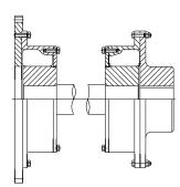
Cardan Shaft Coupling: Used to increase the distance between shaft ends and give a higher misalignment capability.
