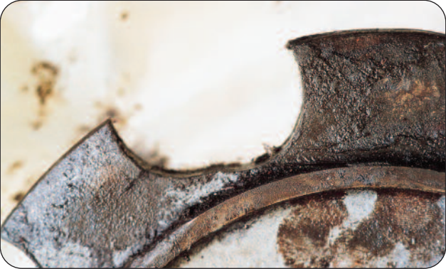
Figure 41 - Mode of Failure - Sprocket tooth wear
