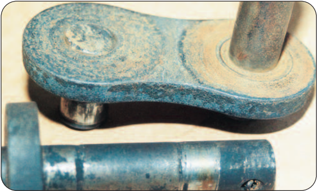
Figure 16 - Mode of Failure - Lubrication & Alignment
