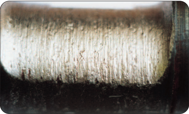
Figure 37 - Mode of Failure - Overheating
