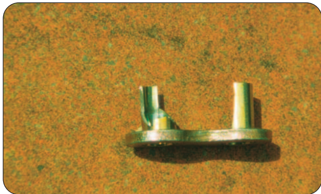
Figure 9 - Mode of Failure - Fracture
