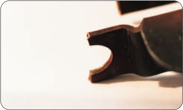
Figure 43 - Mode of Failure - Tensile overload
