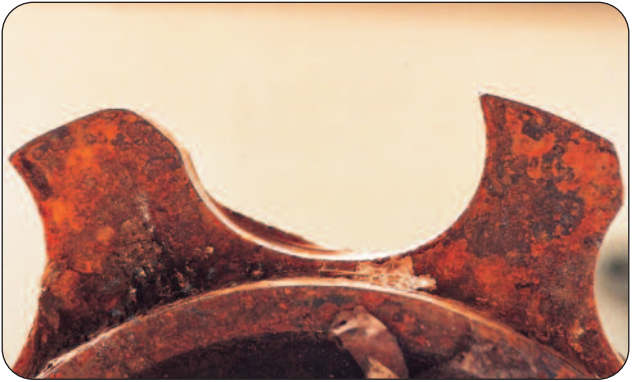
Figure 26 - Mode of Failure - Alignment
