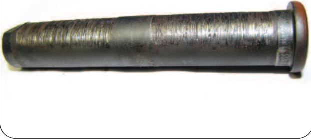
Figure 13 - Mode of Failure - Galling
