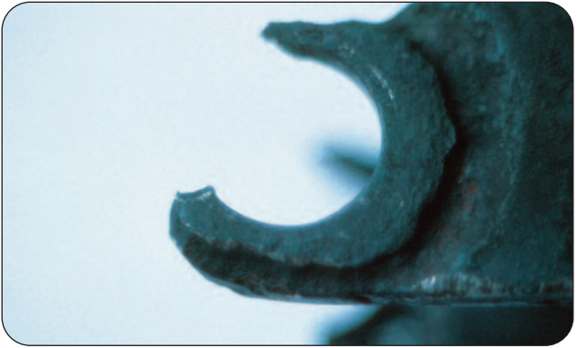
Figure 30 - Mode of Failure - Corrosion/Erosion
