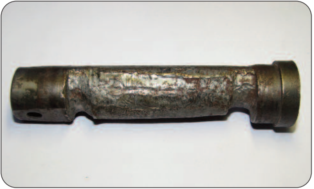
Figure 7 - Mode of Failure - Erosion
