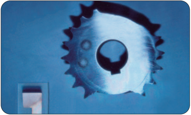
Figure 17 - Mode of Failure - Material cracking below teeth
