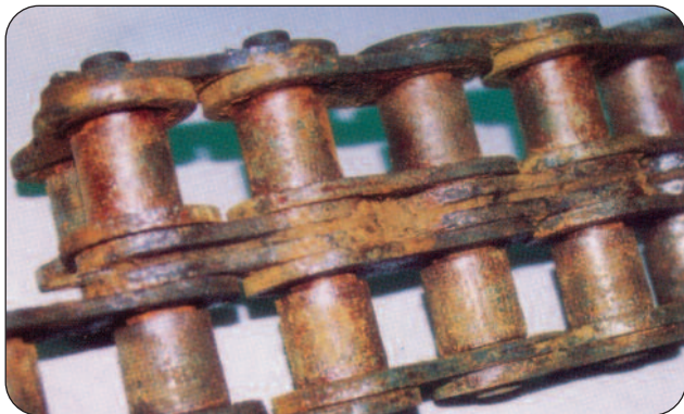
Figure 5 - Mode of Failure - Corrosion/Erosion
