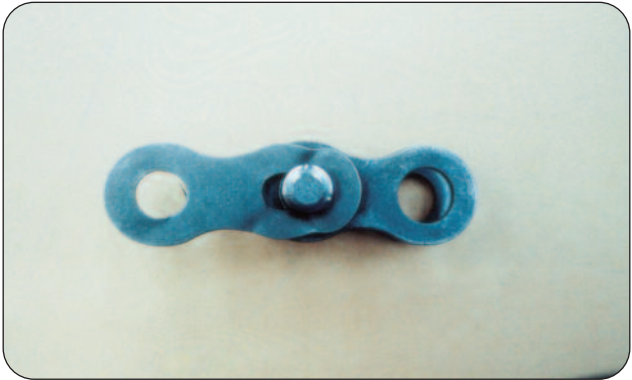
Figure 18 - Mode of Failure - Overload
