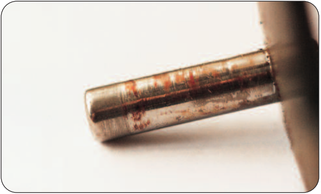
Figure 11 - Mode of Failure - Fretting Corrosion
