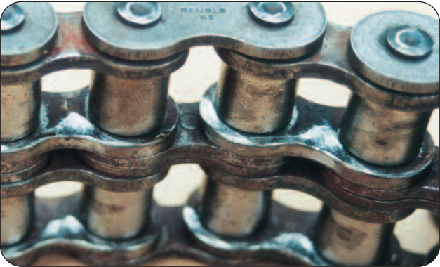
Figure 14 - Mode of Failure - Lubrication & Alignment
