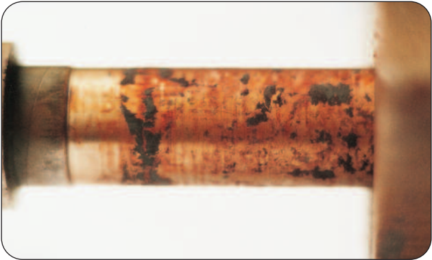
Figure 31 - Mode of Failure - Fretting
