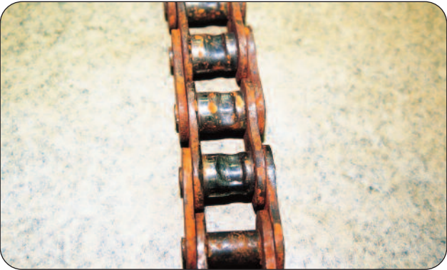
Figure 4 - Mode of Failure - Corrosion
