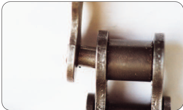
Figure 21 - Mode of Failure - Riveting Failure
