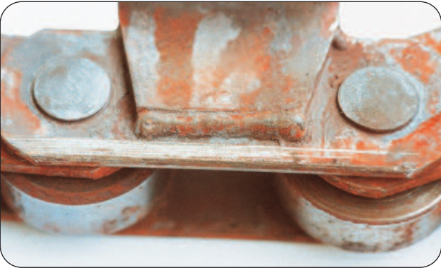
Figure 23 - Mode of Failure - Alignment
