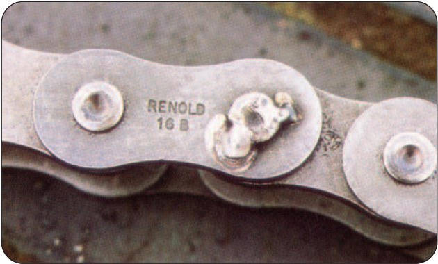
Figure 6 - Mode of Failure - Cracking
