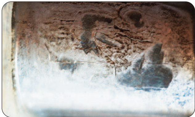
Figure 32 - Mode of Failure - Impact & alignment
