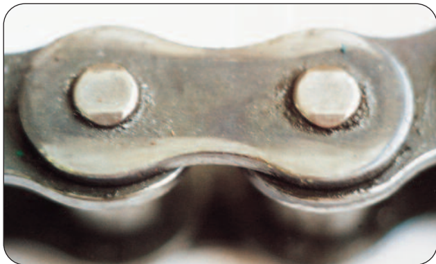
Figure 1 - Mode of Failure - Alignment
