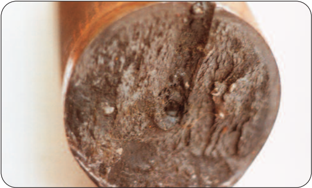
Figure 35 - Mode of Failure - Misalignment
