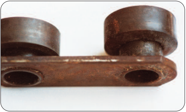
Figure 40 - Mode of Failure - Roller Seizure
