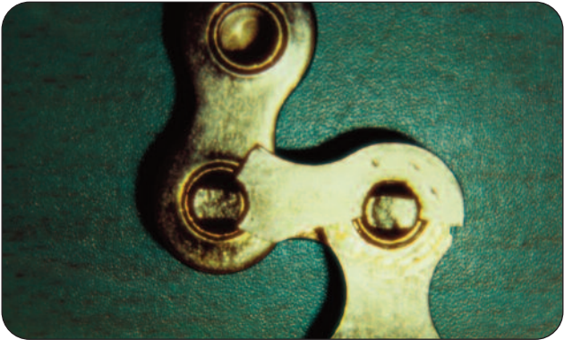
Figure 10 - Mode of Failure - Fracture
