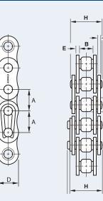
Miniature chains are available in 11SS and are well-suited for lightduty applications in a wide variety of business machines (copiers, printers, vending machines, etc.). The rollerless chains are made entirely of 304 Stainless Steel with bushings riveted in place for superior corrosion and temperature resistance.
