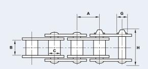
These chains possess the same strength and working load values as standard ANSI chains. They are designed for tension linkage applications such as lifts or hoists and are usually supplied in odd numbers of pitches with a connecting link (drive fit recommended) at each end. Offset links are not recommended for hoist applications. The numbering system for rollerless chain substitutes the number 5 for the number 0 at the end of the corresponding ANSI chain number.
